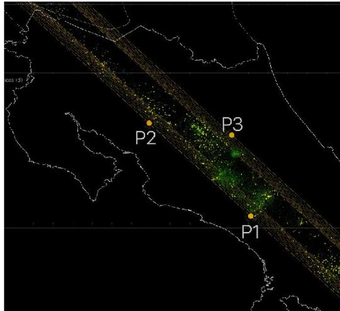
Fig.2 The three points needed to define a seismic profile in Plinius
